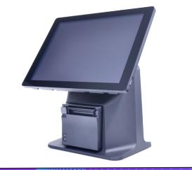
This tablet base includes a printer for the for the lowest profile solution to printing customer receipts.
